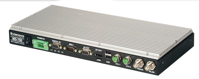
The VIANOVA vehicle server is an on-board computer particularly developed for mobile applications. It is the hardware platform for the VIANOVA software products including passenger information, entertainment, video surveillance and passenger counting. The system performance is more than sufficient to run all these applications simultaneously with reserve.
